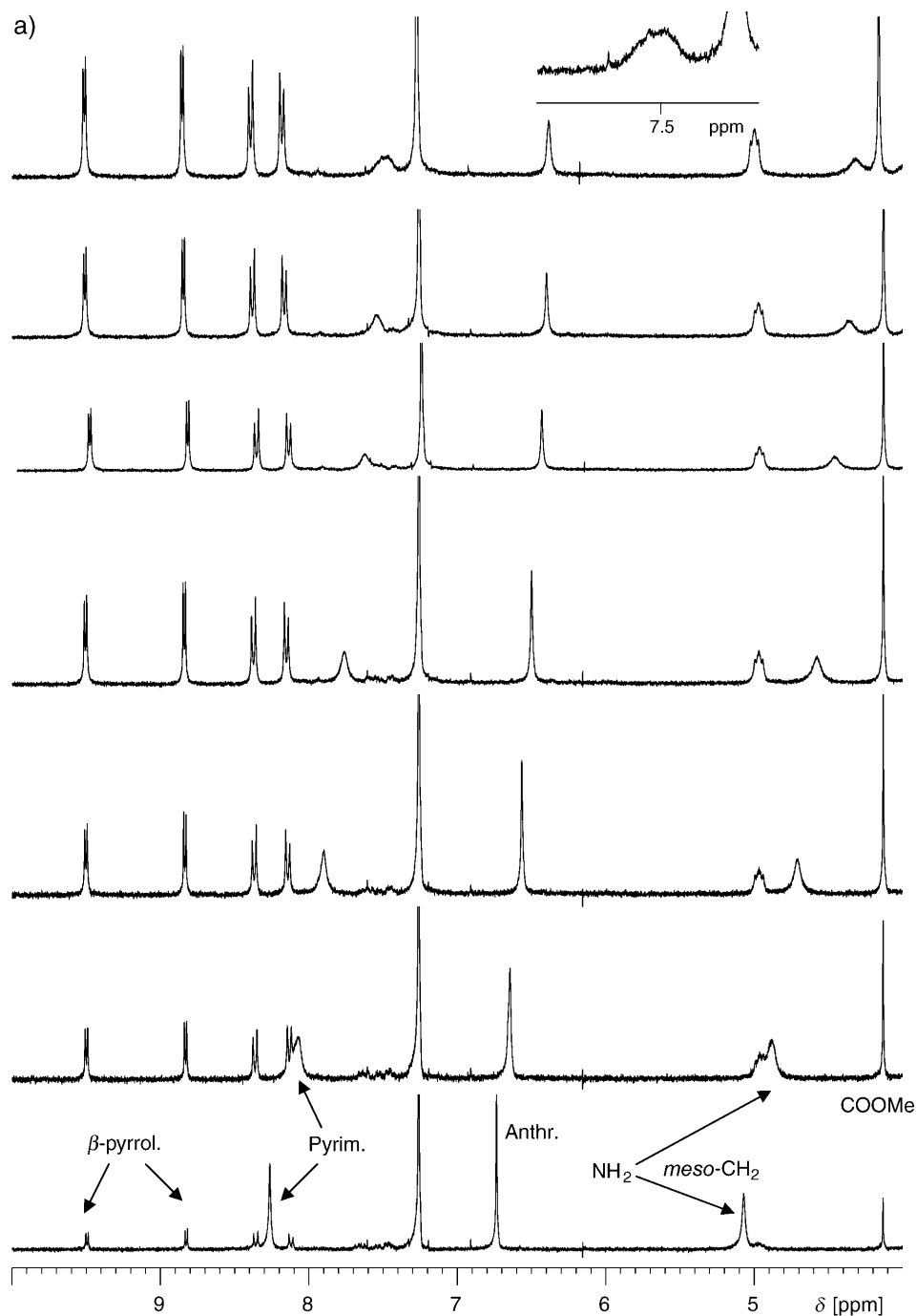
Fig. 5. a) Low-field region of the ^1\text{H-NMR} spectra (300 MHz, \text{CDCl}_3 , 25^\circ ) of 6 upon addition of porphyrin 19 . b) Temperature dependence of the low-field ^1\text{H-NMR} region (300 MHz, \text{CDCl}_3 ) at a 1:1 stoichiometry between 6 and 19 . Note that the pyrimidine-proton signals, which show a broad and partially complicated splitting at 25^\circ , sharpen and shift to lower field at 35^\circ , but there is hardly any change from 45 to 55^\circ .
